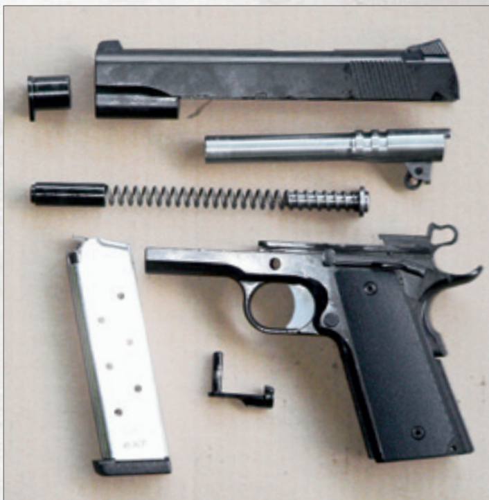
The Valor pistol disassembled for routine maintenance
