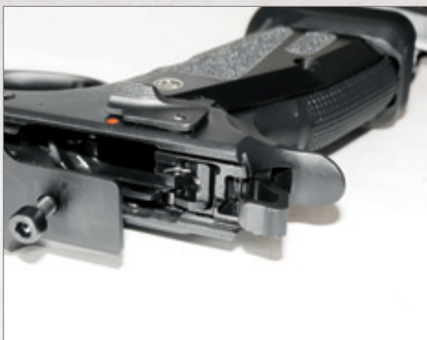
Single action firing and trigger mechanism of the CZ 75 TS CZECHMATE
