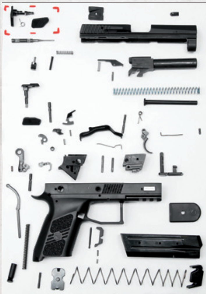
Complete disassembly of the CZ 75 P-07 DUTY. The red window in the top left corner shows parts necessary for replacement of the safety with the decocking lever.
