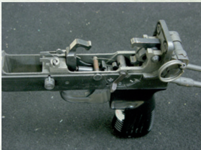
The trigger and firing mechanisms and the rate-reducer of the CZ SKORPION 9x19
