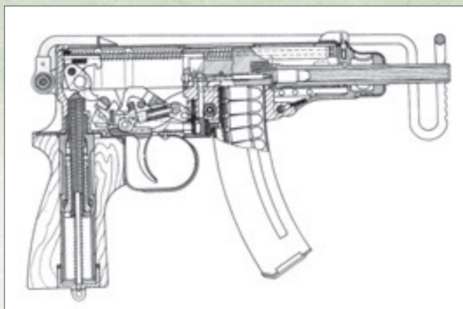
Cross-section of the Skorpion development prototype (S-59). It differs from the S-61 serial model by its fixed rear sight and non-removable shoulder stock.
