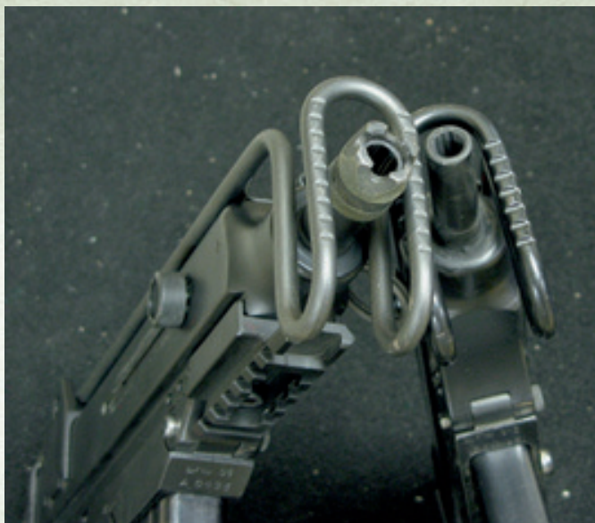
Comparison of the Skorpion muzzles in calibers 9 mm Luger and 7.65 Browning. The CZ SKORPION 9x19 dated from 2001 on the left; vz. 61 E from 1992 on the right.
