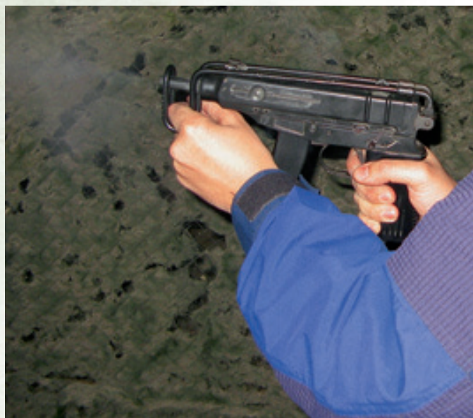
The 61 E submachine gun from the small production series originating in 1992 from aside: the user can hold the butt of the folded stock with the non-shooting hand to support the gun.
