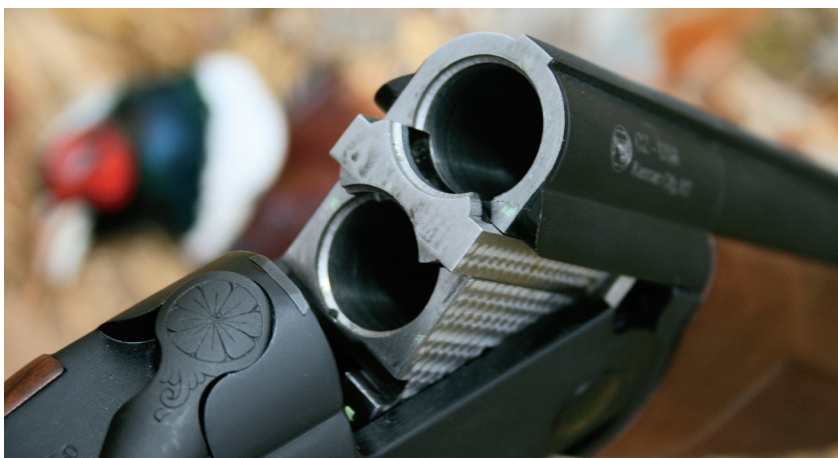
A single beefy double-sided extractor muscled out hulls with no difficulties. Tolerances in the action were superb.
