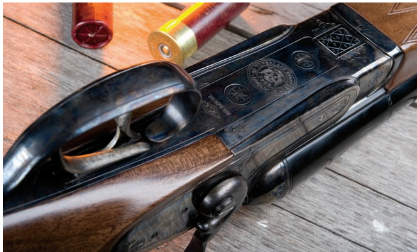
Having aligned screw slots allows you to tell at a glance if one is backing out.
